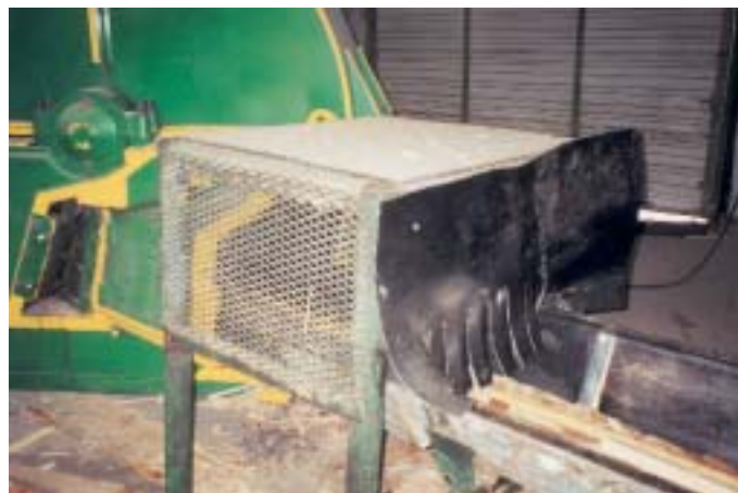
Fig. 2: Fringed rubber strip (from old conveyor belt) stops wood scraps that chipper occasionally deflects backward.
