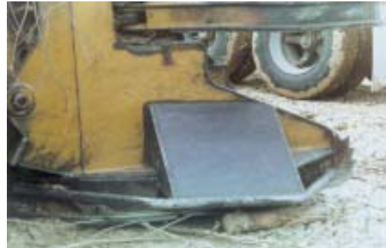
Fig. 1: This homemade deflector was retrofitted/welded on an old sawhead model.
