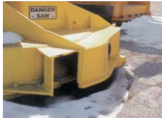
Fig. 3: Newer Timberjack sawhead shows how debris on a Timberjack/Waratah-installed retrofit is deflected through two right-angle turns. Timberjack believes this is a better alternative to the homemade, downward-facing deflector.
