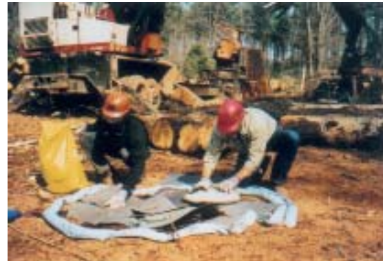
Fig. 1: Most spill kits contain "socks," which help contain a spill, and ultra-absorbent pads or pillows.
